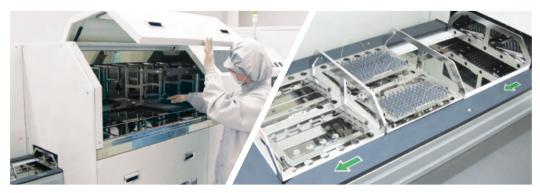
The cleansing process by ultrasonic wave using the 3rd distilled water, vacuum dry, and heating dry sterilization leaves no residue and ultimately sterilizes the products.
