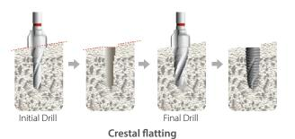
> Use the crestal cutter of the Initial Drill and Final Drill. > Longer drill than fixture's length can be used as well.
